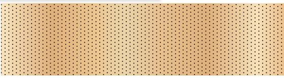
0.5 mm perforations spaced 2mm O.C. vertically and horizontally
