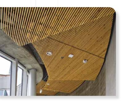
ACGI Grille Systems feature two categories—Grille Backer Series (GB) and Grille Dowel Series (GD). Both systems are available in solid wood or wood veneer (depending on blade size and design requirements). Blade sizes are typically 1%"–3½" deep (for depths greater than 3½" see our Baffle Systems). Grille panels are typically assembled with four to ten blades per foot. Panels are nominal 1' or 2' width by varying lengths in 1' increments (custom widths and lengths are available).
