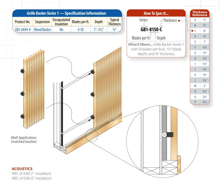
Grille panels are a traditional product offering the warmth of wood plus acoustical treatment. A large amount of open area allows sound to pass unobstructed into the plenum space and/or acoustic insulation behind the panels. Consequently, acoustical performance of a wood grille is determined by the properties of the absorbing medium. This medium is often fiberglass insulation in bags, mats, or duct liner.
